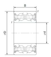
40 mm x 62 mm x 20,625 mm NSK 40BD49 angular contact ball bearings
